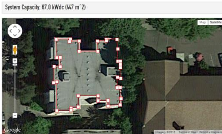
Figure 15. Roof and usable PV areas estimation (Ref. NREL-PV Watts)
